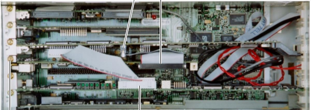
⑤ Remove the faceplate screw from slot 3 with the screwdriver provided, then remove the optional line interface.
