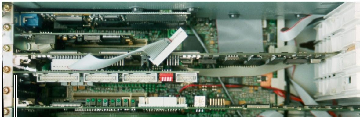
② Install the ARIB interface card into slot 3 and screw the faceplate to the PC chassis. (If this is the first interface installed into slot 3, you will have to remove the blank faceplate first.)
