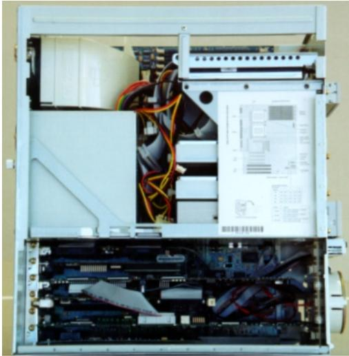
⑥ If your optional line interface is connected to the MPEGscope main card with a cable, disconnect the other end of the cable from the MPEGscope main card and remove the cable.
