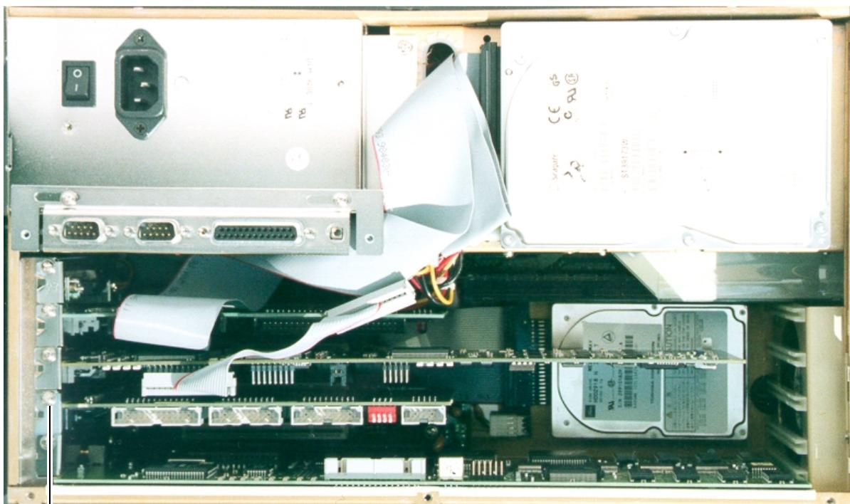
② Install the ARIB interface card into slot 2 and screw the faceplate to the PC chassis. (If this is the first interface installed into slot 2, you will have to remove the blank faceplate first.)
