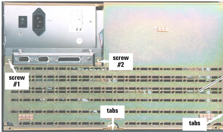
① Insert tabs on the sides of the metal shield into the slots on the outer frame, then replace the two metal shield screws.
