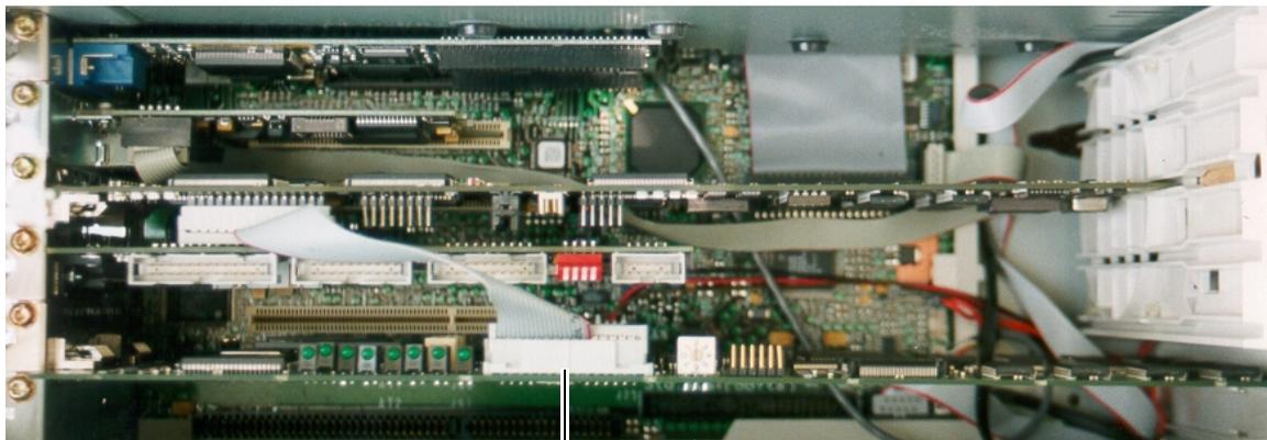
③ If your MPEGscope has a Real-time Analyzer, reconnect the ribbon cable from the MPEGscope main card to the Real-time Analyzer card.
