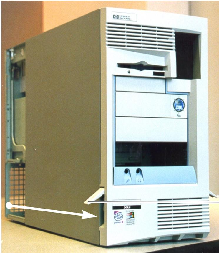
⑤ Flip the two latches on the front sides of the computer cover upwards.
