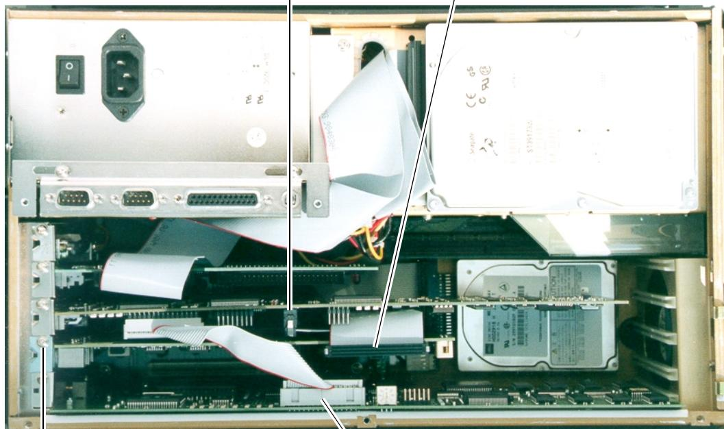
④ Remove the faceplate screw from slot 2 with the screwdriver provided, then remove the optional line interface.
